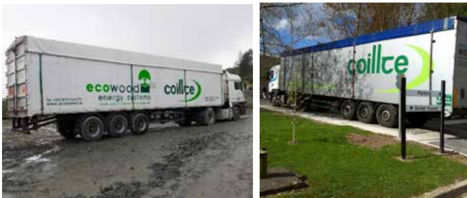
Figure 5: Biomass haulage. Image shows moving floor trailer deliveries to an industrial scale boiler. Trailers typically carry 20 to 24 t and can off-loaded at the client's fuel store in about 15 minutes.
