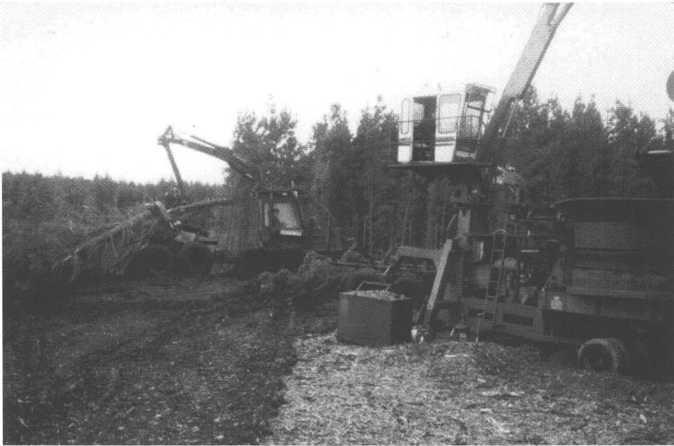
Figure 2. The whole tree chipping site at Oughterard, Co. Galway. The system involves a Manitowoc delimeter/debarker, a Morbark chipper, and a Barkbuster.
