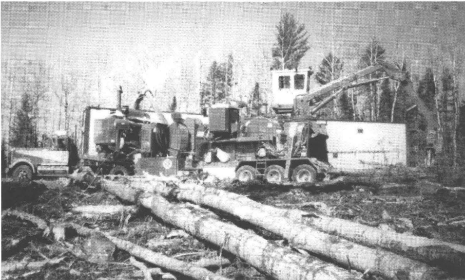
Figure 4. A Morbark Total Harvester in operation in north-western Ontario, Canada. This machine is capable of producing 100 m 3 of chips per hour, and represents state-of-the-art technology in relation to whole tree chipping.
