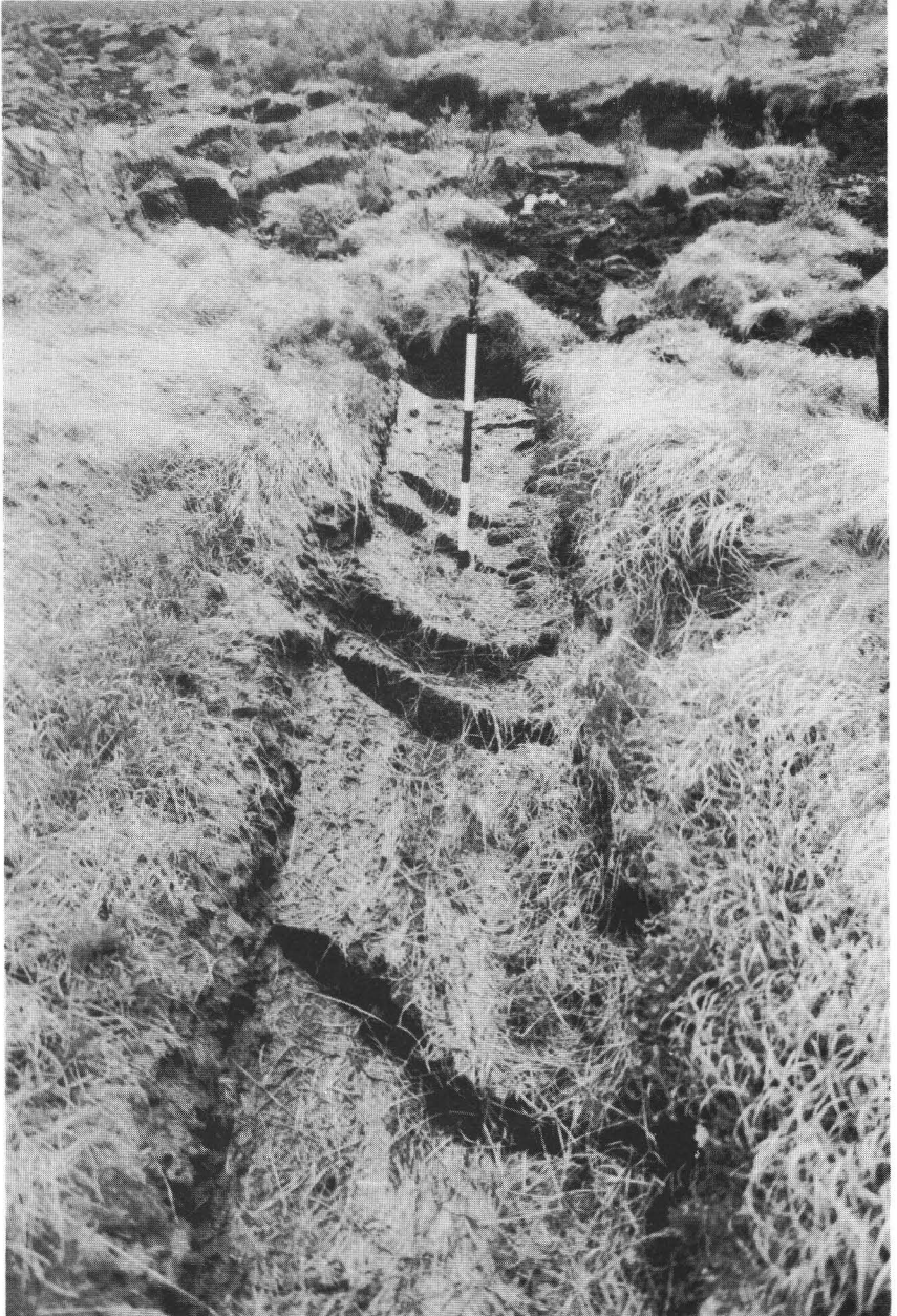
Figure 7: Lateral tears in bottom of DMB furrow immediately above head of flow.
