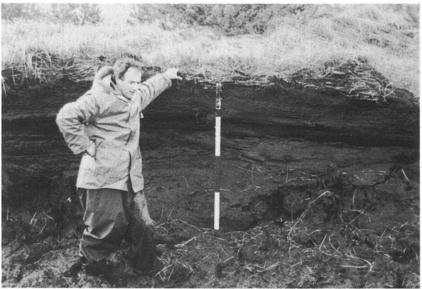
Figure 4: Peat depth about 1.7m (near forest road) – rod is 1.5m high and is resting on bog floor.
