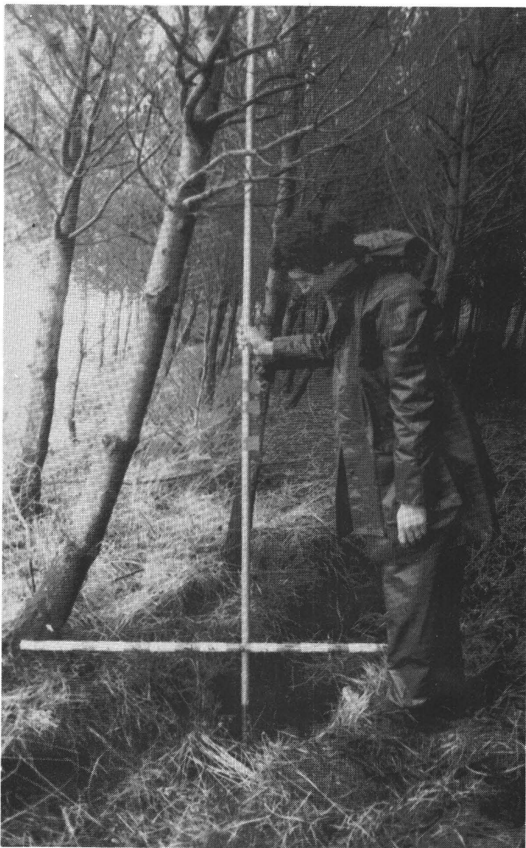
Fig 2. Method of measuring maximum stem deviation from the vertical.
