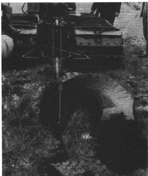
Fig. 1 Tunnel plough in operation at Glenamoy, Co. Mayo.
