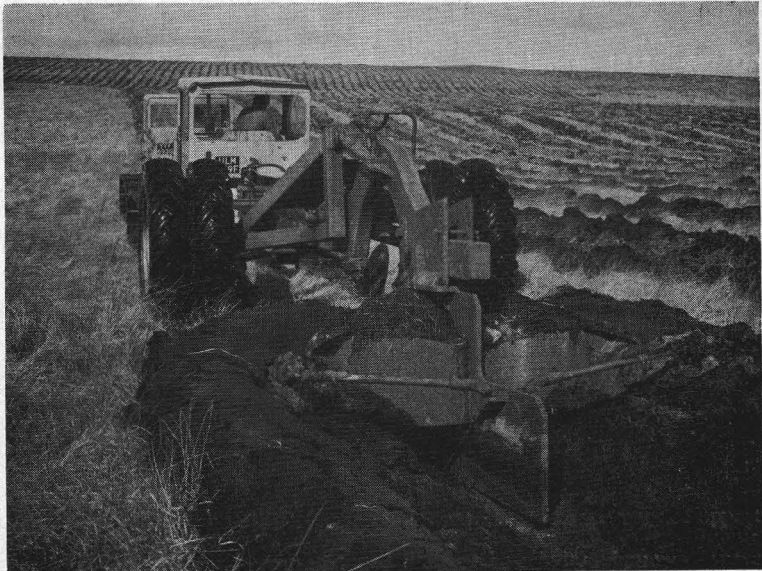
Figure 2: Parkgate/Humpy deep double mouldboard tine plough for planting on peat.
