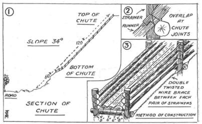
joined by a "scarf" or overlap joint to prevent fouling by the descending logs. The heavy side runners were "shouldered" against the uprights. As far as possible, runner poles were joined at and wired to the cross-pieces. Light poles were used as side rails to prevent the skidding logs from "jumping" the chute.
