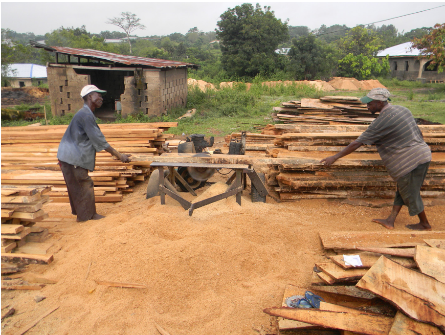
Figure 7: Waste generation in Nigerian sawmills: a large portion of this material is used as fuelwood and for poultry bedding, while most of the sawdust is incinerated.
