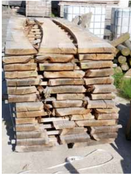
Figure 8: E. nitens rough-sawn planks at Dundrum sawmill.
