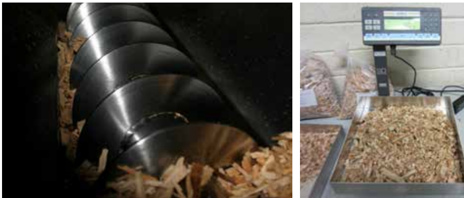
Figure 4: Panel A shows a wood chip auger infed to an industrial biomass boiler for steam production. Panel B shows part of the routine quality testing procedures employed to ensure the quality parameters of supply lots. Variation in quality parameters (moisture and others) can be high so processing plants rely greatly on the knowledge and experience of contractors to help ensure that a consistently high quality product is supplied.
