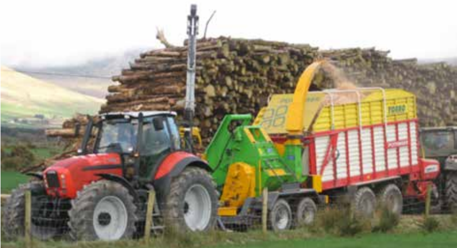
Figure 2: Biomass wood chip production at Coillte's biomass processing hub in Caherciveen, Co. Kerry.
