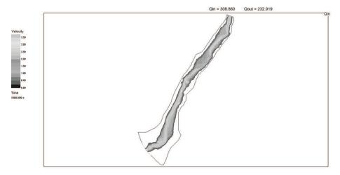
Figure 15: Modelled velocity distribution  $(ms^{-1})$  across Floodplain 3 at and around the peak of the flood for dense woodland. Qin and Qout are inflow and outflow rates in  $m^3 sec^{-1}$ .
