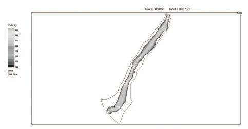
Figure 16: Modelled velocity distribution  $(ms^{-1})$  across Floodplain 3 at and around the peak of the flood for grassland. Qin and Qout are inflow and outflow rates in  $m^3 sec^{-1}$ .
