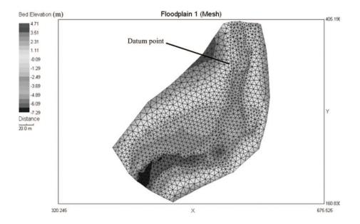
Figure 7: Shaded topographical representation (relative to the datum point) of Floodplain 1 with the overlying computational mesh. Datum point indicates 0 elevation of topographical data.
