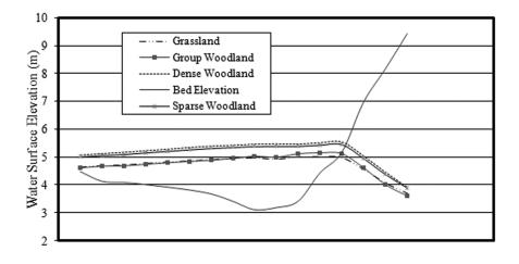
Figure 12: Modelled water surface elevations above OD at cross section 4 at the peak of the flood for the four vegetation scenarios in Floodplain 3. See Figure 8 for cross section location.
