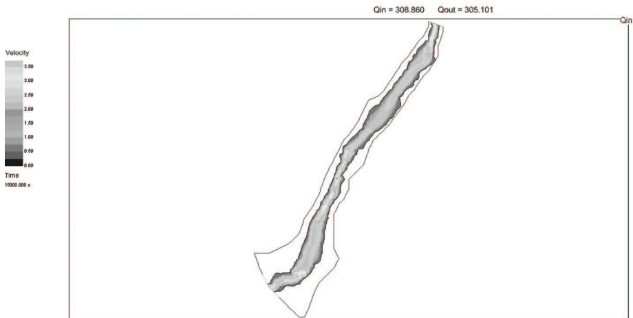
Figure 16: Modelled velocity distribution ( \text{ms}^{-1} ) across Floodplain 3 at and around the peak of the flood for grassland. Q_{in} and Q_{out} are inflow and outflow rates in \text{m}^3\text{sec}^{-1} .
