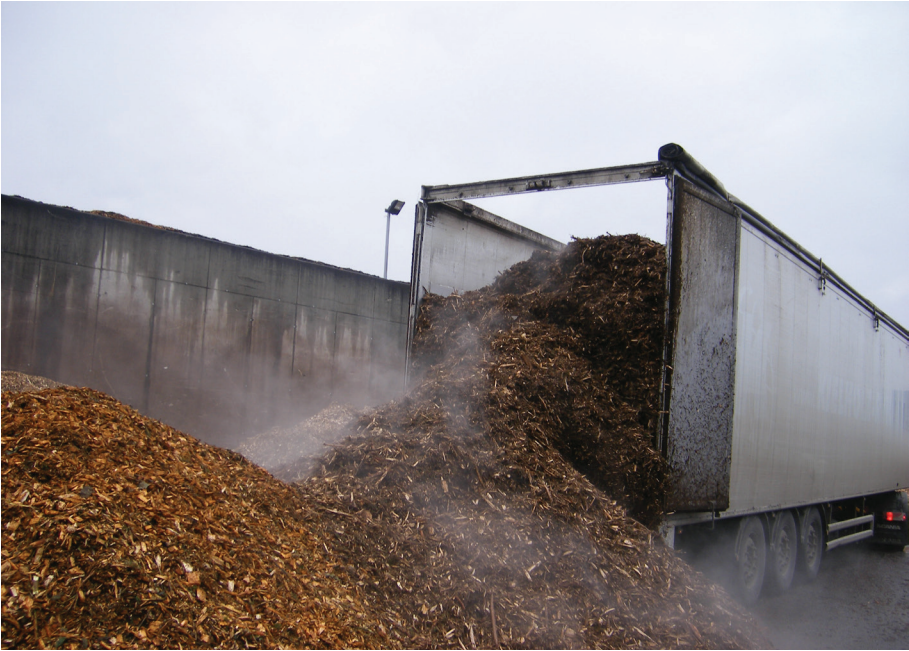
Figure 3: A truck load of steaming chips arrives at the Rastensfeld biomass power plant which is operated by Nawaro-Energie GmbH. As loads will vary in calorific value and ash content, the chips are mixed thoroughly in the yard before being fed into the furnace.
