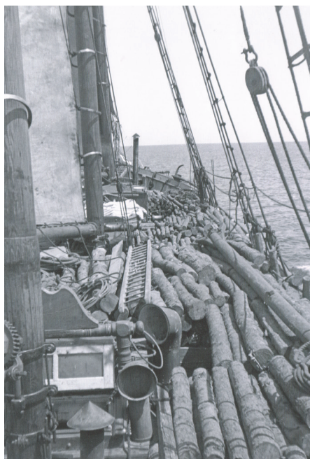
Figure 3: Agnes Craig loading pit props at Headboro on the Bride River (near Youghal), August 1948. Note the use of the cargo gaff and tackle to lift the logs on board. Photograph courtesy of Richard J. Scott.
