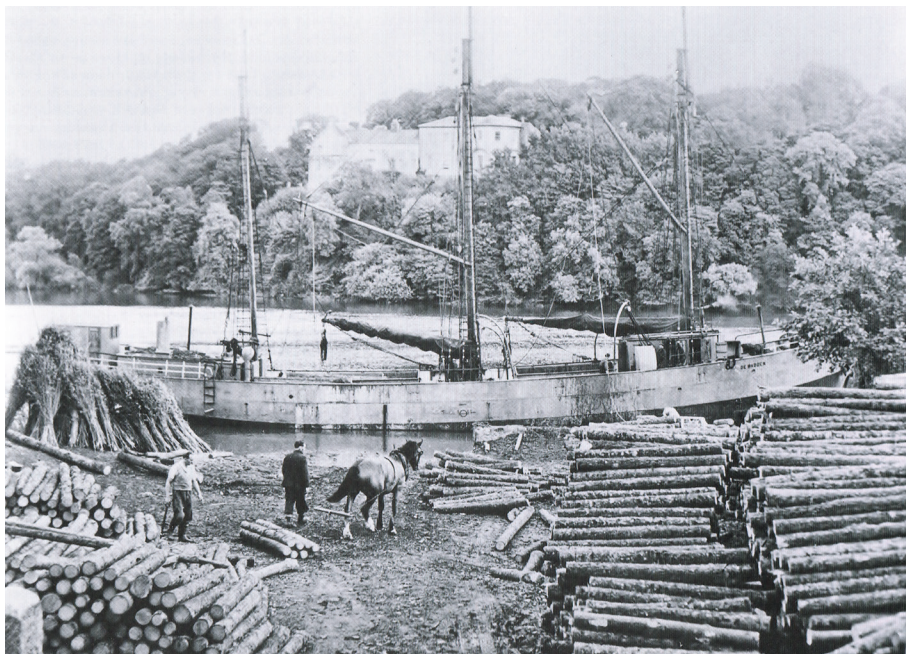
Figure 2: Kathleen and May bound for Newport with the last cargo of pit props from Ballinacurra to the Bristol Channel in June 1960. Note the holds are full and the remainder of the cargo is on deck, making work for the crew difficult, and the temporary safety line rigged between the shrouds offered little protection. The long spar on top of the timber is a heavy gaff, specifically for cargo work. Photograph courtesy of the National Maritime Museum.
